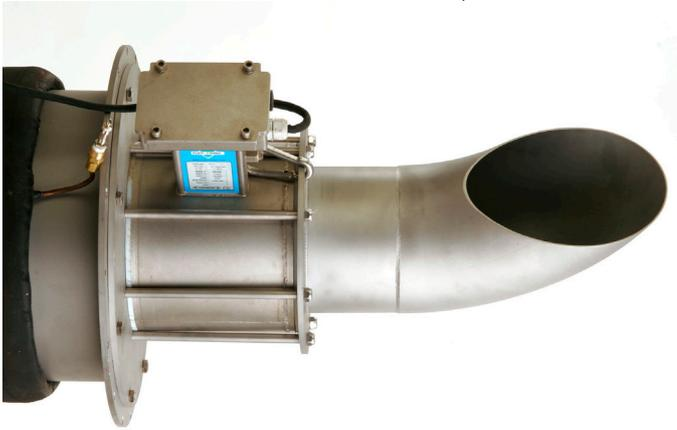
The SEWER-MAG™ is an insertable full bore electromagnetic flow meter sensor. It ensures extremely accurate flow determination even under difficult flow conditions. The Sewer-Mag is usually temporarily installed in sewer networks to verify or calibrate existing flow meters.
